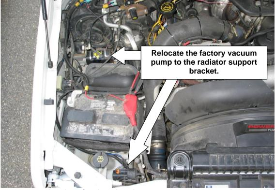
Cut the power supply wires for the electric vacuum pump approximately 4" from the connector and splice in the black and blue wires supplied using the butt connectors and shrink tubing. Route the relocation loom along the fender and towards the front up to the new vacuum pump location. Inside of the loom should be the supplied black and blue wires, along with the 1/8" plastic vacuum tube. Shrink tubing has been provided to securely seal these connections.
