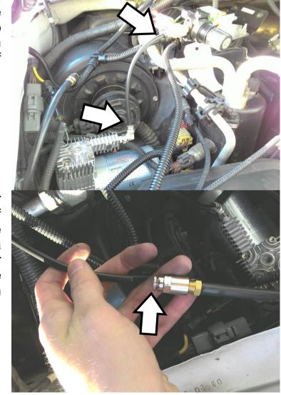
Install the intake air filter for the air compressor by adding a length of 1/4" air tubing to the rubber hose section. Then route this 1/4" line to a dry location (behind the regulator assembly is suggested). Install the "pancake" style filter supplied with the pump to the end of this tube.
