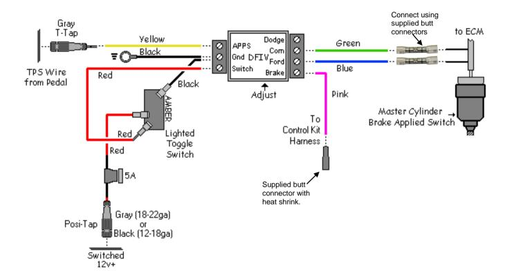
Remove lower section of dash, under the steering column, and mount the DFIV module to the cross member under the steering column. Connect the Black wire from the DFIV module to a good ground.
