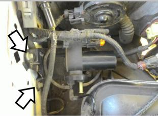
Remove the small electric vacuum pump from the stock bracket by removing the screws. Reinstall on to the supplied relocation bracket. Trim the rubber ends on the three vibration dampers to clear when reinstalling. Install on the passenger side of the radiator support bracket with the two bolts and washers provided.
