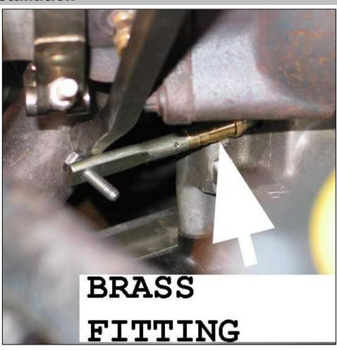
downwards to expose the valve actuation rod.
