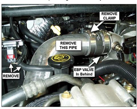
When removing the pipe, the lower rubber boot that connects to the intercooler should remain on the pipe. The pipe slides out of the rubber boot that is still attached to the intake manifold.
